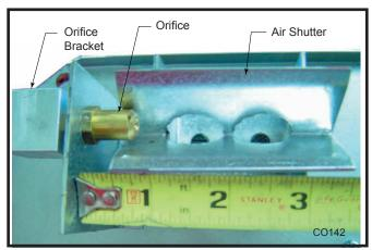
**Fig. 15** The air shutter setting is 1/2" (13 mm) from the orifice bracket to the edge of the air shutter.
